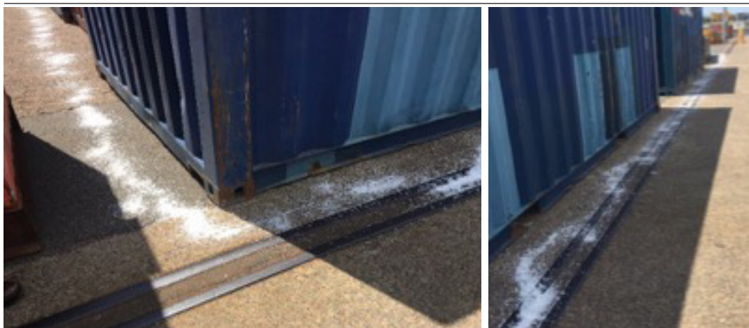
FIGURE 8 Ring-salting around segregated CAL containers awaiting inspection
