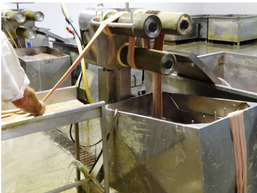
Figure 7 Separation of mucosa and threads from sheep intestines on a stripper/crusher machine, Australia
