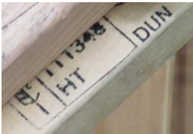
Figure 7 Unacceptable ISPM15 stamp—obscured by timber nailed over it
