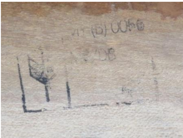
Figure 5 Unacceptable ISPM 15 stamp—incomplete and illegible through poor printing
