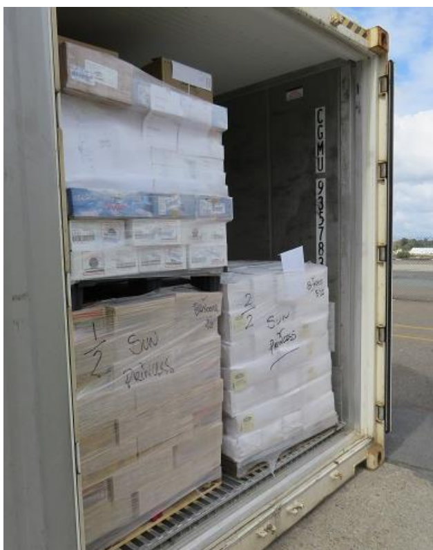
Figure 9 Full container load, demonstrating limited access for inspection of timber packaging
