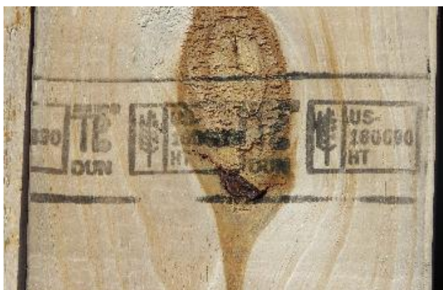
Figure 8 Acceptable ISPM 15 stamp—continuous and legible
