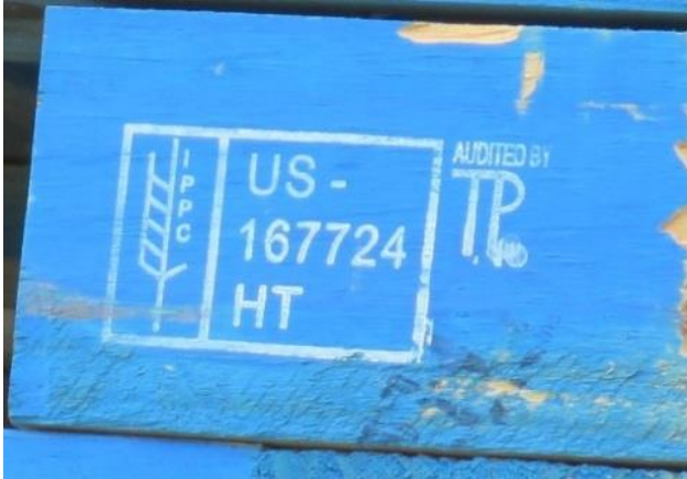
Figure 4 Acceptable ISPM 15 stamp—complete and legible
