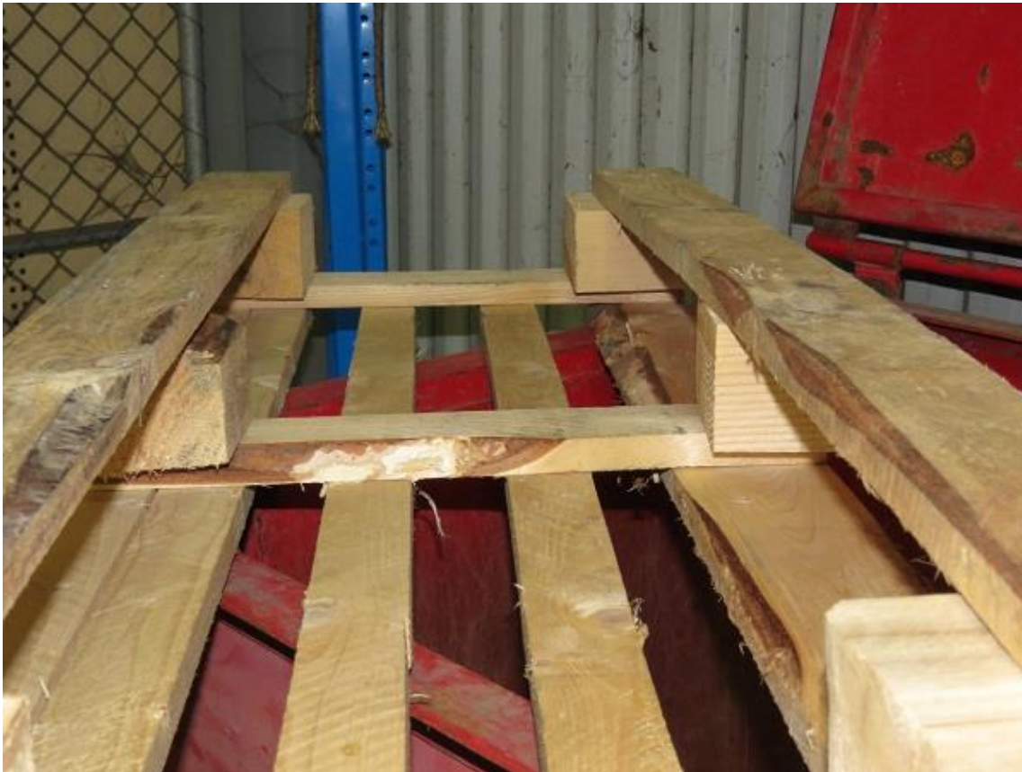
Figure 1 Timber pallet with bark contamination exceeding ISPM 15 tolerance
