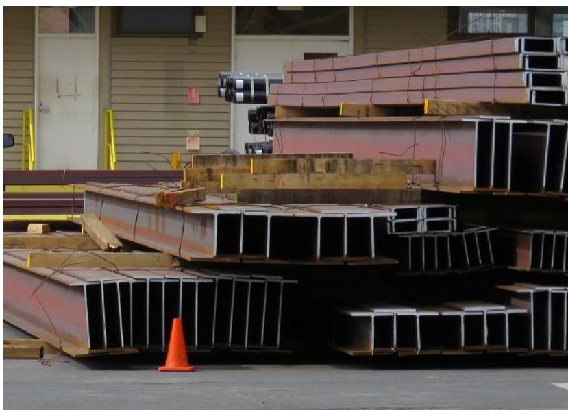
Figure 9 Break bulk cargo—steel beams stacked on timber dunnage at a wharf
