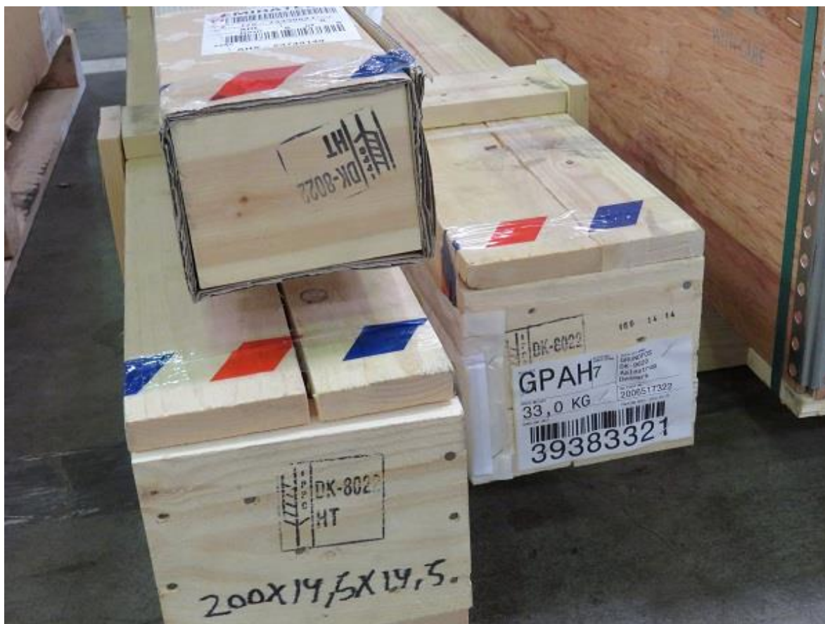
Figure 3 Wooden crates with ISPM 15 stamps correctly applied to each crate
